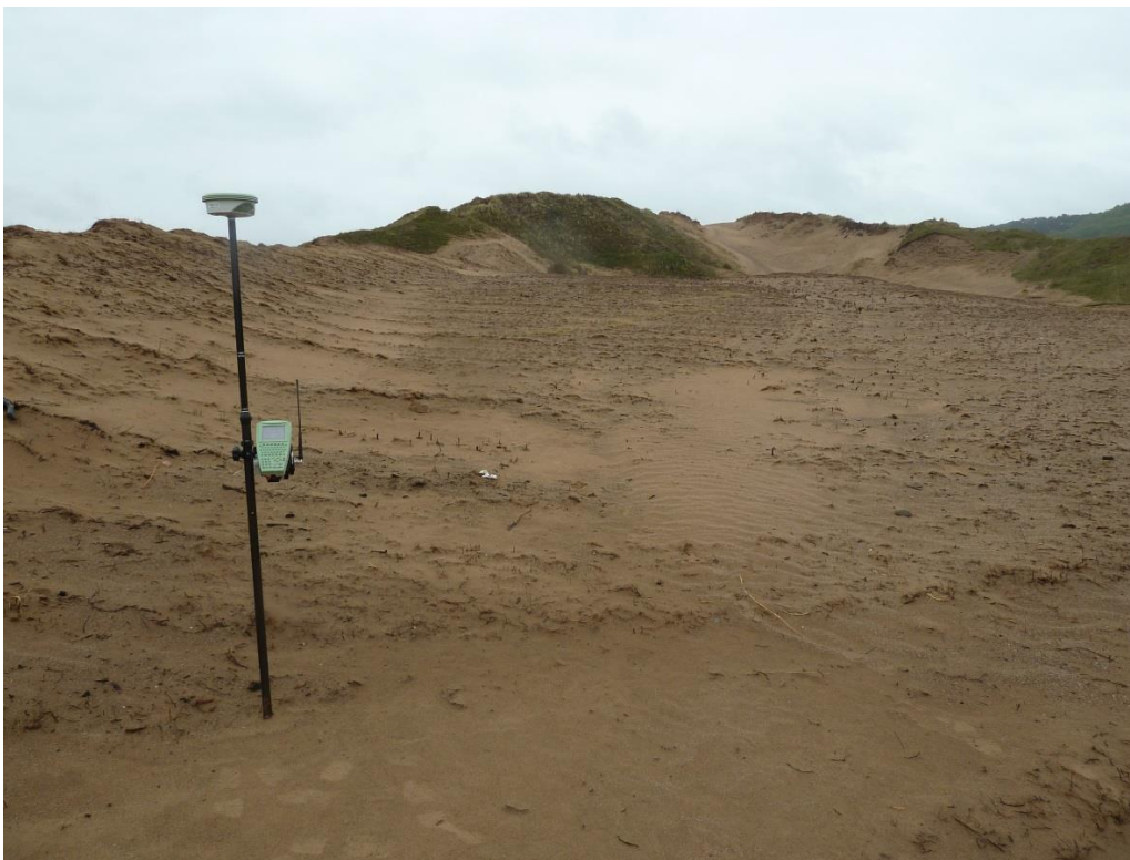
Photo 12. Vegetation and sand stripping on the north side of the site have produced a pronounced plateau. SmartRover surveying equipment in the foreground.
