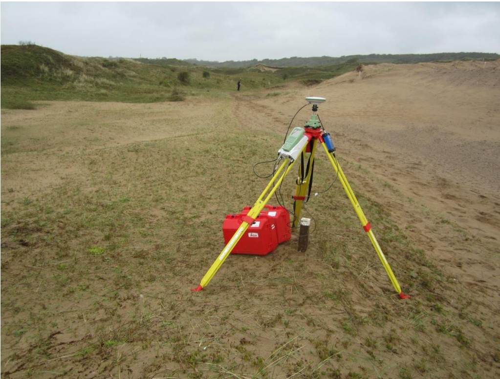
Photo 13. Survey base station, set up over Benchmark 1
