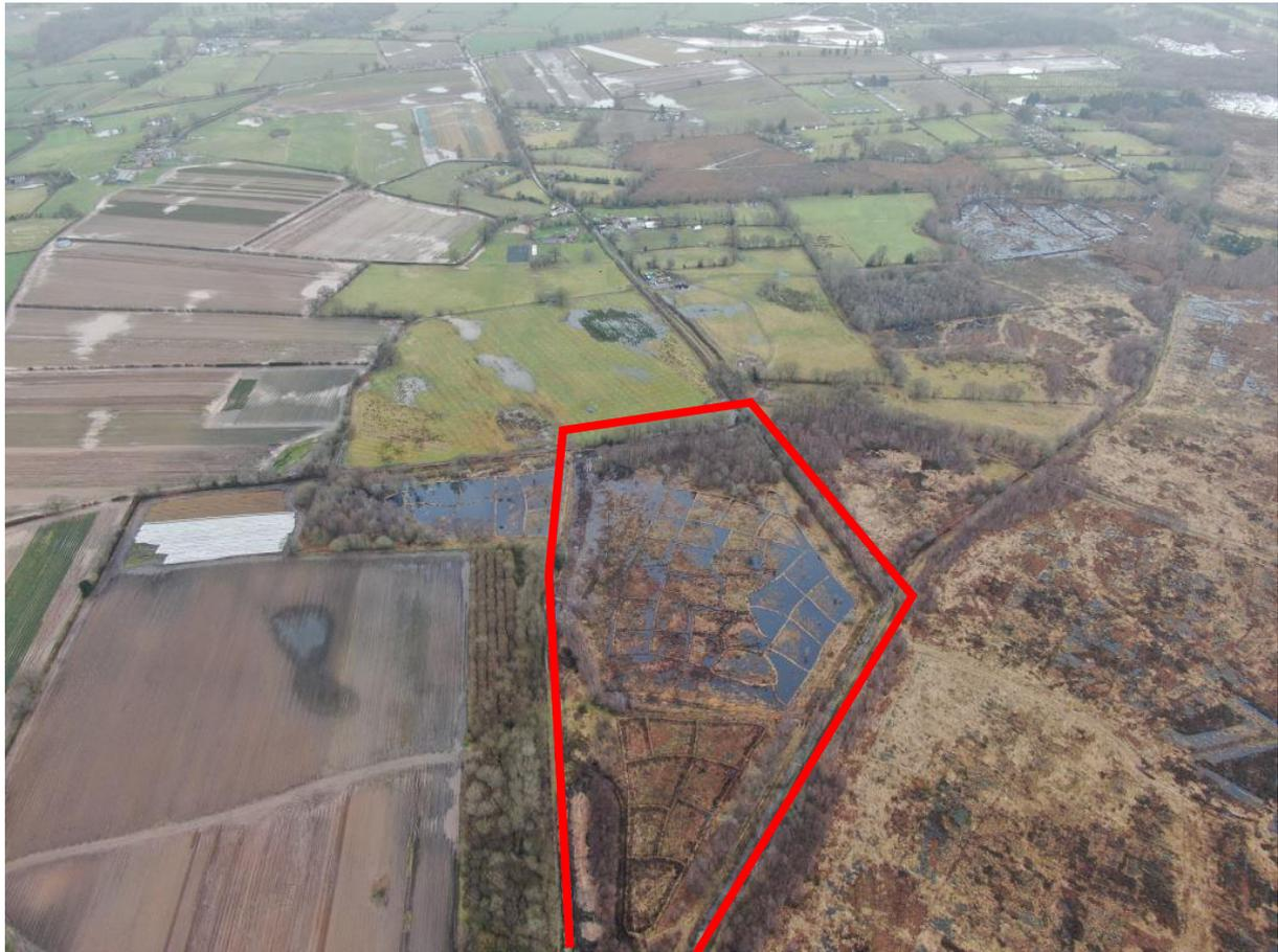
**Figure 7.** Low contour bunding cells installed with NPAP funding in compartment 33 of the Fenn's, Whixall, Bettisfield, Wem & Cadney Mosses SAC during 2020-2021. This site is the third largest lowland raised bog in the UK and work there contributes to the NPAP Lowland Peatlands Priority Action Theme.
