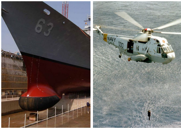
Left: Hull-mounted AN/SQS-53 series MFAS on the USS Cowpens; source: Wikipedia Commons . Right: AN/AQS-13 series dipping sonar (MFAS) deployed from a helicopter; source: Wikipedia Commons .
